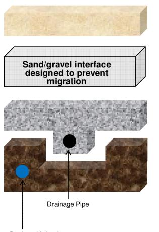
Modified sand profile consisting of sand and fibre mix
